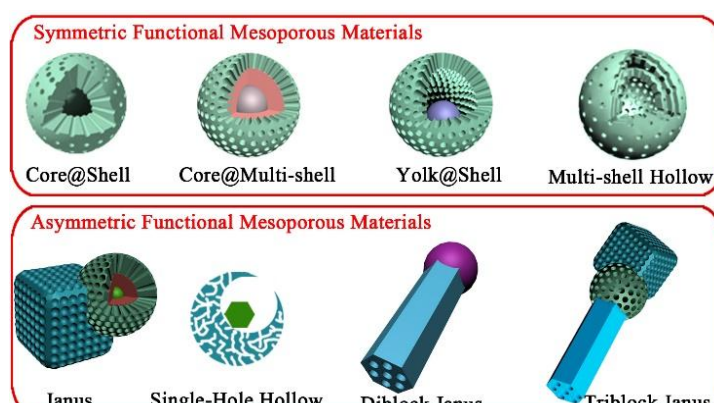
Fig. 1: Scheme illustration of the symmetric and asymmetric functional mesoporous materials.
